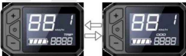
Press the "M" button to navigate through the menu and obtain the information. ODO record. Trip distance. ONLY MEASURE kilometre by kilometre.
