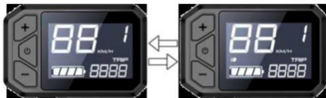
Pressing the "+" button twice with the display on switches from Km/h to Mp/h and pressing the "-" button twice switches from Mp/h to Km/h.
